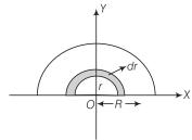
(a) The half-disc can be supposed to be consists of a large number of semicircular rings of mass dm and thickness dr and radii ranging from r = 0 to r = R.
