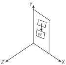
A force can produce torque only along a direction normal to itself as  $\tau = \mathbf{r} \times \mathbf{F}$ . So, when the door is in the xy-plane, the torque produced by gravity can only be along  $\pm z$  direction, never about an axis passing through y-direction.
